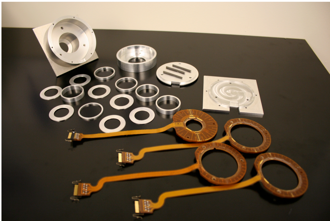
Figure 3.19: REPTile EM disassembled to show individual components.
